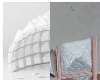
7. INSERTED POLYSTYRENE FOAM PYRAMIDES CUT BY ROBOT
