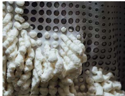
2. STRETCHED FABRIC + POLYURETHANE
