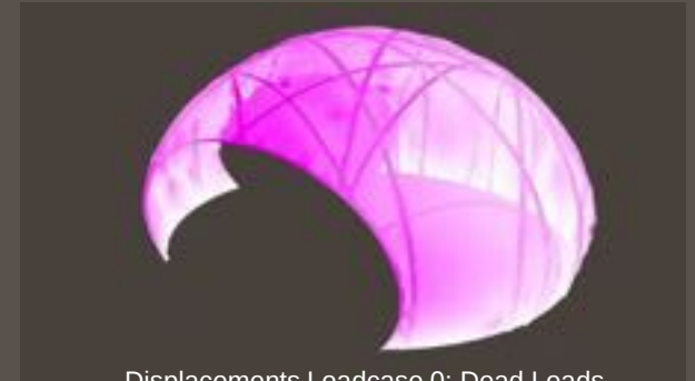
Displacements Loadcase 0: Dead Loads
